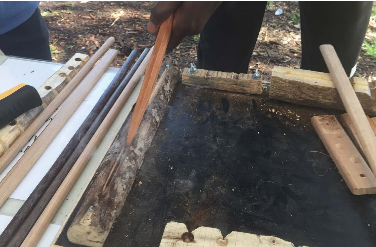
A fire plough illustrates conversion of kinetic energy to heat energy
